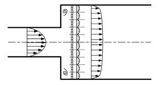
2 Fig. 2. Schematic view of the effect of perforated baffle on the homogenization of velocity profile.
