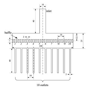
4 Fig. 6. Geometry and dimension of the numerical benchmark (unit: mm).
