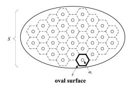
2 Fig. 20. Division of a baffle surface by numerous control volumes for 3D application.
