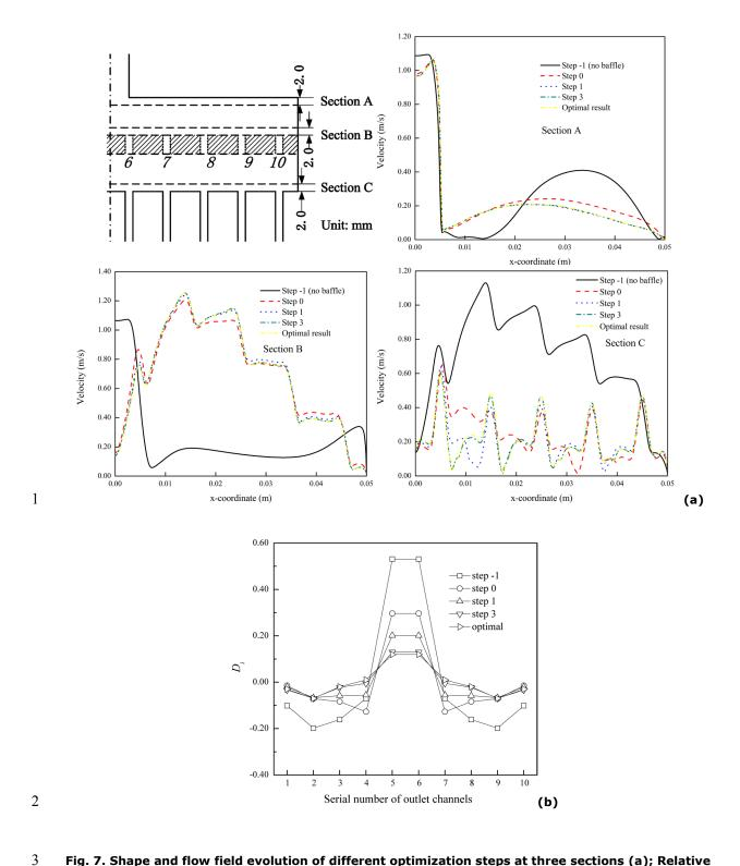
Fig. 7. Shape and flow field evolution of different optimization steps at three sections (a); Relative
