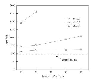
7 Fig. 19. Influences of global porosity and number of orifices on the pressure drop increase. M=10;
