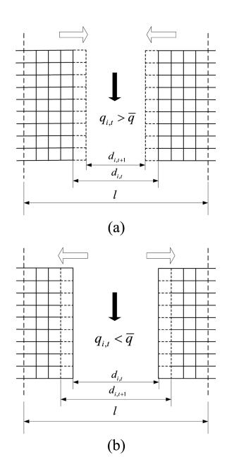
**Fig. 4. Basic principles of the optimization algorithm.** (a) Reduction of the orifice; (b) Enlargement of the
