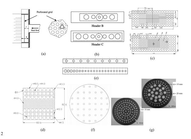
3 Fig. 1. Different baffle configurations proposed in the literature. (a) Adapted from Lalot et al. (1999). (b)
