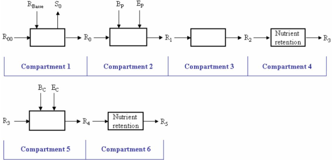
**Figure 2.** Model structure, where, R is a sampling point into the Têt River or La Basse tributary, S refers to the Têt water taking, B is the WWTPs' bypass, E is the WWTPs' effluent, P refers to the Perpignan's WWTP and C refers to the Canet-en-Roussillon's WWTP.
