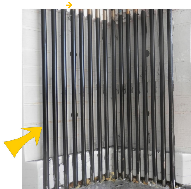
Figure 1. 3D view of the pilot multi-tube solar receiver (Credit: PROMES-CNRS), with solar cavity, refractory lined; and 16 parallel UBFB receiver tubes; → concentrated solar irradiance flux.
