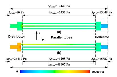
Figure 12: Pressure drop values on different parts of the solar receiver (Inconel 600 as filling material): (a) without baffle insertion: (b) with optimized baffle insertion.
