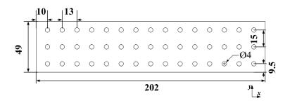
Figure 4: Geometry and dimensions of the initial (uniform) perforated baffle for optimization (unit: mm).
