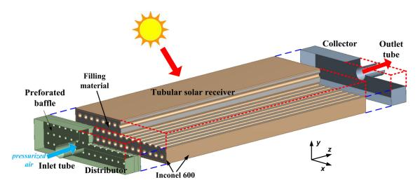
Figure 1: Schematic view of the tubular solar receiver equipped with an inlet fluid distributor and an outlet fluid collector.
