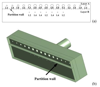
Figure 10: Optimized baffled fluid distributor for the tubular solar receiver when Inconel 600 is used as the filling material: (a) optimized baffle configuration (diameter, unit: mm); (b) distributor geometry.
