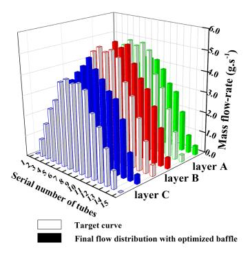
Figure 6: Comparison between the final flow distribution with optimized baffle and the target curve (copper as the filling material).
