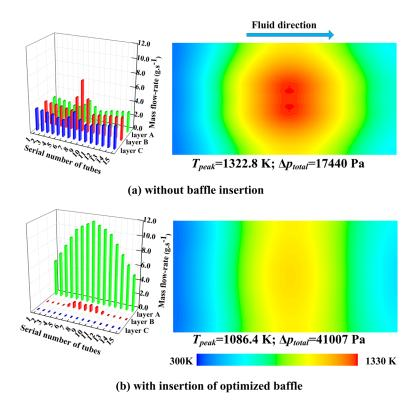
Figure 11: Fluid flow distribution among parallel tubes and the corresponding temperature field of the heated surface (Inconel 600 as the filling material): (a) without baffle insertion; (b) with insertion of optimized baffle.
