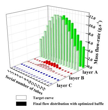
Figure 9: Comparison between the final flow distribution with optimized baffle and the target curve (Inconel 600 as the filling material).
