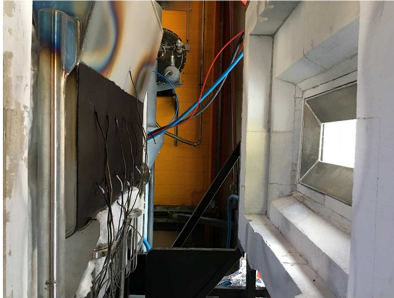
Figure 6. View of the reactor (left) inside the cavity with the welded thermocouple on the front wall. Right side is the water-cooled aperture and the inner insulation.
